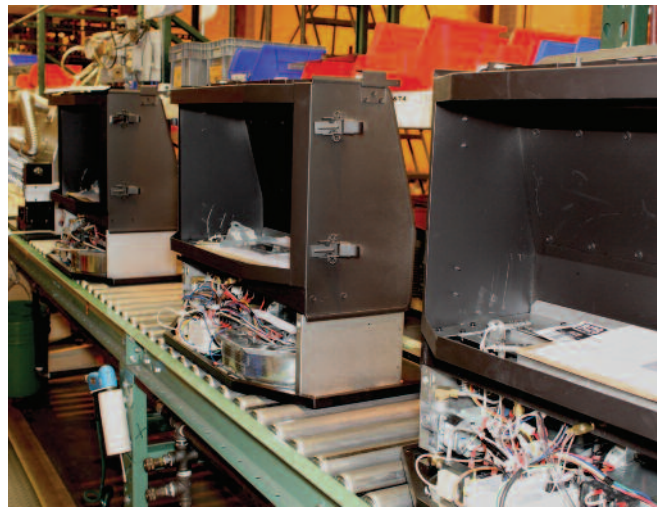
Mantis fireplaces undergo preparation for the final assembly line at Empire. Mantis is a 90%-plus efficient fireplace.
