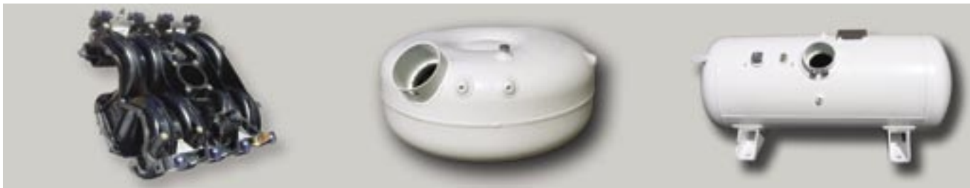
Roush's F-150 LPI fuel rail assembly features two fuel rails, an insulated crossover, and a service port. Fuel storage choices include a 20-gal. toroidal tank that fits between the rear frame rails and an optional 50-gal. in-bed tank.
